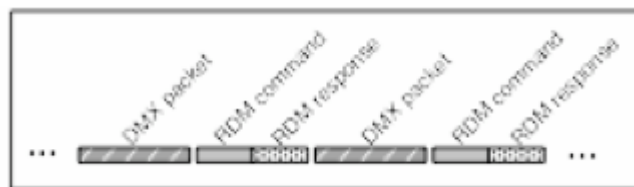
DMX and RDM Signal Packet Diagram
